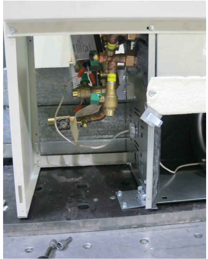
FIG. 9 - FRONT CLIPS ATTACHED TO UNPAINTED SHEET-METAL FRAME
